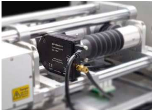
Optional onboard camera available to monitor beam profile, pointing and pulse to pulse stability
