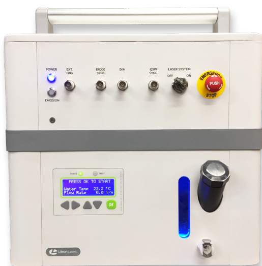
Free standing PSU and chiller (separate units)
