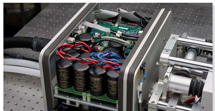
Power supply for pump diodes located inside laser head
