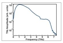
**Tera-SED3** emission spectrum at 10 V DC bias and 0.7 nj pulse energy, acquired with Laser Quantum GmbH (formerly Gigaoptics) ' High-Speed ASOPS technique.
