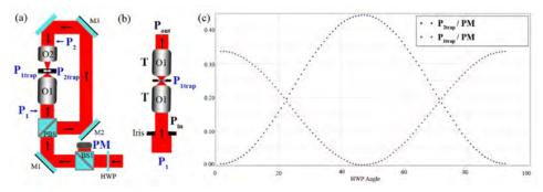
Fig. 9. Procedures to calibrate the laser power at the trapping position. (a) Laser power check points. (b) Measure the laser transmission of the objective lens. (c) The calibrated curve for the laser power at the trapping position.
