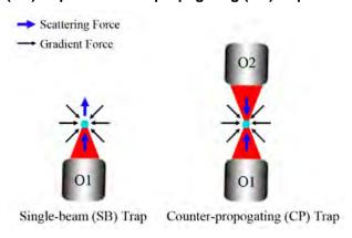
Fig. 1. Compare single-beam and counter-propagating trap.
