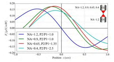
Fig. 3. Calculated optical force along laser propagating direction (z direction) for a 200 nm GNP in CP trap. The NA of the lower objective lens O1 is NA = 1.2, the NA of the upper objective lens O2 changes from NA = 1.2 to NA = 0.4. P2/P1 is the power ratio between the upper and the lower beam.
