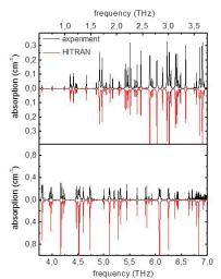
Figure 2: THz absorption of water vapor compared to data compiled from the HITRAN database. Agreement below ~2.5THz is excellent with dynamic range limitations to the peak height at higher frequencies. Total measurement time was 1 minute
