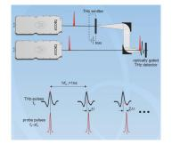
Figure 1: Optical layout of ASOPS based THz-TDS experiment. One laser pulse train pumps an emitter of THz radiation, the second probes the THz pulses in an optically gated detector (after interaction with a sample). As result of the repetition rate offset, the probe laser samples different advancing data points of the signal with each pulse pair.
