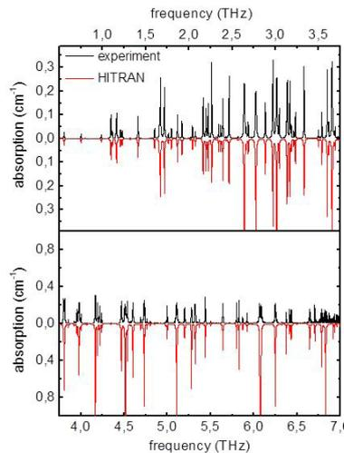
Figure 2: THz absorption of water vapor compared to data compiled from the HITRAN database. Agreement below  $\sim 2.5$  THz is excellent with dynamic range limitations to the peak height at higher frequencies. Total measurement time was 1 minute.
