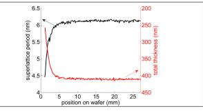
Fig. 4. The superlattice period and total superlattice thickness of the Si/Mo mirror with respect to the distance from the wafer edge. Results show layer thickness decrease at the mirror edge.
