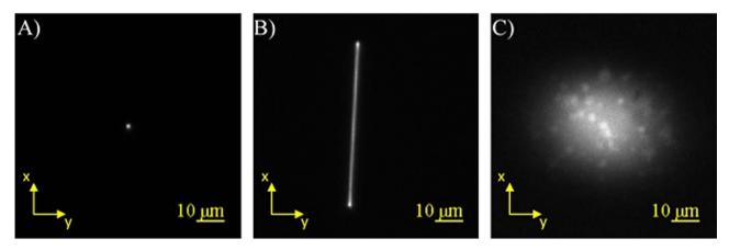
Figure 2. Characterization of the tightly-focused and relaxed Gaussian beams. (A) Normalized image of fluorescence from a QD film showing the beam profile of a tightly focused Gaussian beam. (B) Normalized image of the tightly focused Gaussian beam being scanned across a QD film. (C) Normalized image of a relaxed Gaussian beam exciting the same QD film. Spots in the image are due to imperfections in the QD film.
