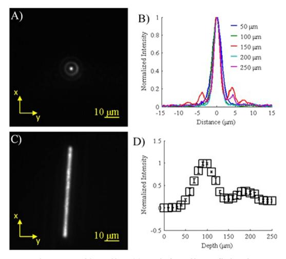
Figure 1. Characterization of the Bessel beam. (A) Example of a Bessel beam profile obtained using a QD film ( $z=150\,\mu m$ ). (B) Normalized plots of the Bessel beam profile for various depths along the z-axis. (C) Image of the Bessel beam being scanned where the exposure time is much longer than the scanning period. (D) Relative intensities of the Bessel beam along the z-axis (n=5, error bars represent standard deviation).
