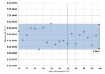
Fig. 1 Typical wavelength stability versus head temperature of torus laser.
