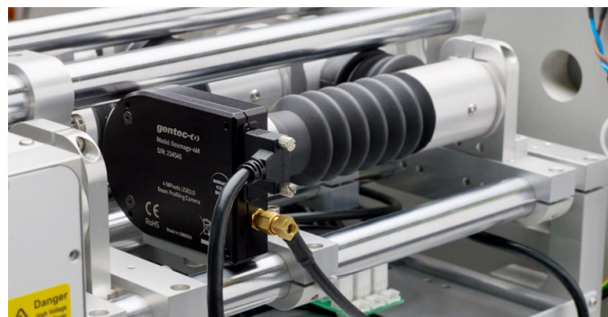
Real time beam profile monitoring option
