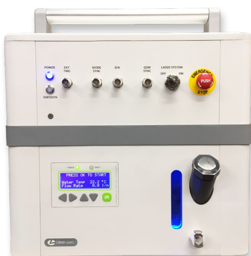
Free standing PSU and chiller (separate units)
